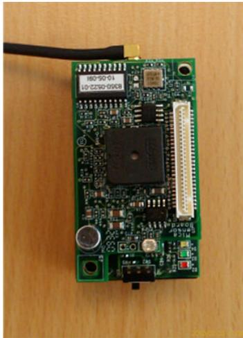
**Fig. 3** Multisensor radio module for device monitoring
